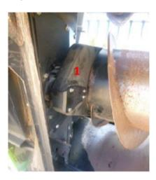
Step 2: loosen and remove idler chain sprocket
