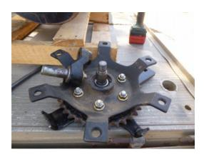
Step 11: Remove LH Mount Arm off Sprocket Hub:
