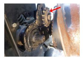
Step 3: Remove endless drive chain
