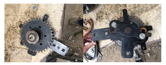
Step 8: Remove LH end out of Drum by removing the 6 Bolts from around the outside:
