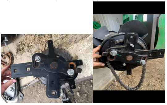
Step 13: Fit Mount Arm Assembly to Turbodrum with 6 Bolts from OEM sprocket:
